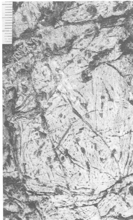
Fig. 11: Interlocking bladed aggregates of calcite defining a spinifex texture. Upper section of north-west gully. Scale bar in cm.
