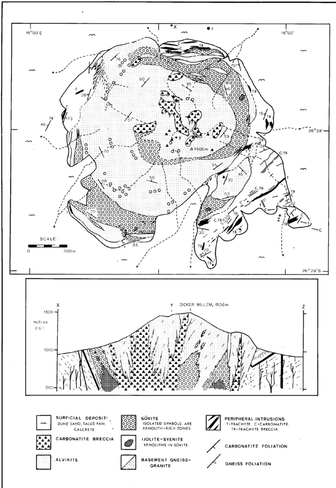
Fig. 1: Simplified geological map and cross section of the Dicker Willem carbonatite complex, south-west Namibia.
